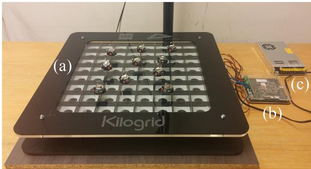
Fig. 1: Picture of the Kilogrid system: (a) Kilogrid of  $8 \times 8$  cells (i.e.,  $4 \times 4$  modules of  $2 \times 2$  cells each) with 10 Kilobots on its Plexiglas surface; (b) the dispatcher that interfaces the Kilogrid with a PC; and (c) the power supply.
