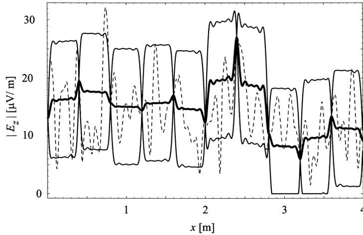
**Figure 6.** Kriging applied to the data set of Figure 1. Kriging estimator (thick line), confidence interval (solid lines), and experimental values (dashed line).
