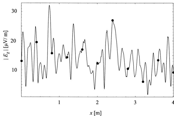
**Figure 1.** Experimental  $|E_z|$  values, and data set (dots) considered for kriging in Figure 6.
