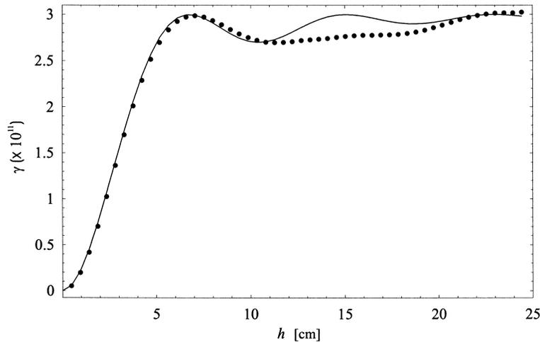
**Figure 3.** Theoretical (solid line) and experimental (dotted line) variograms corresponding to the data of Figure 1.
