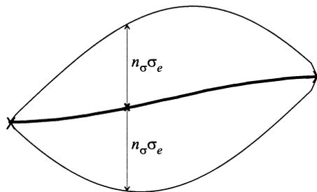
**Figure 4.** Typical kriging result between two known values (crosses). Kriging estimator  $\hat{z}(x)$  (thick line) and confidence interval  $[\hat{z}(x) - n_\sigma \sigma_e(x), \hat{z}(x) + n_\sigma \sigma_e(x)]$  (solid lines).
