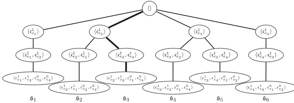
Fig. 2. The complete search tree defined by the solution construction mechanism of the ACO algorithm and the problem instance `kct_simple_inst`. The bold path in the search tree shows the steps of constructing solution  $s_3 = \langle c_{e_2}^1, c_{e_3}^1, c_{e_1}^0, c_{e_4}^0 \rangle$ . Figure from [3]. © Akademische Verlagsgesellschaft Aka GmbH.
