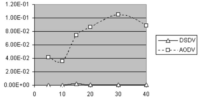
Fig. 6. End to end delay vs. the number of nodes on office's floor (raytracing).
