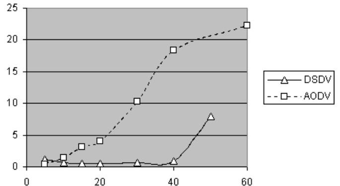
Fig. 7. Routing load vs. the number of nodes (raytracing).
