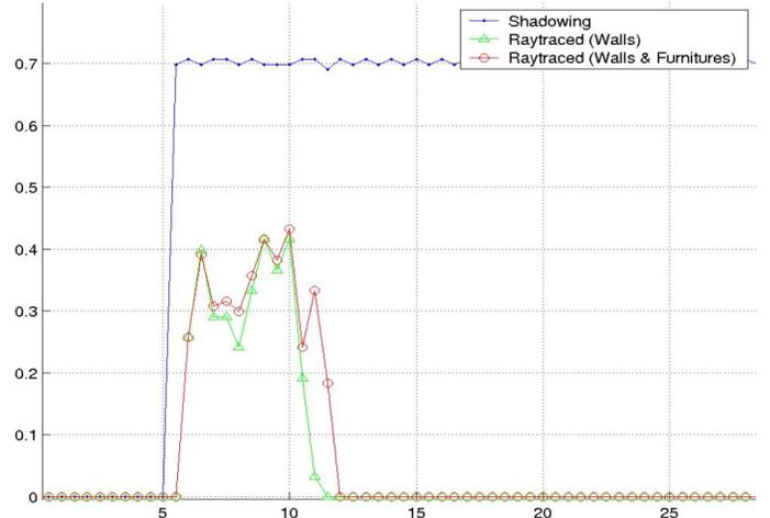
Fig. 3. MAC throughput. Emitter located on (1m,1m), receiver moves away to (30m,30m) with 1m/s speed. Communication starts at t=5s.
