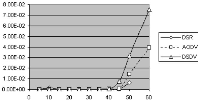
Fig. 4. End to end delay vs. the number of nodes on office floor (shadowing).
