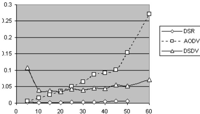
Fig. 5. Routing load vs. the number of nodes (shadowing).
