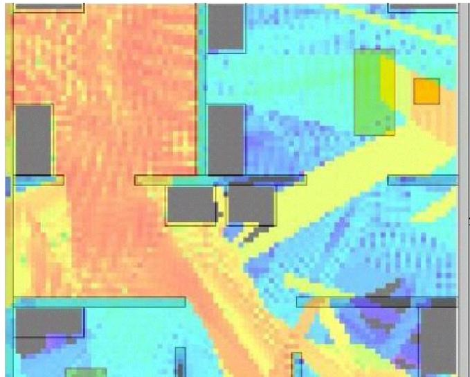
Fig. 2. Field resulting of emitter located on (1m,1m)
