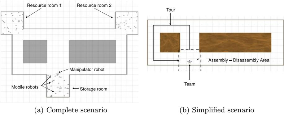
**Fig. 3.** Test task. Figure (a) shows a complete view of the scenario. A swarm of robots must collect as many objects as possible within some time limit from the two resource rooms. Figure (b) shows a simplified version of the scenario. Robots must choose between making the left or right tour. The simplified scenario allows us to concentrate on the decision-making aspect of the task. See text for more information.
