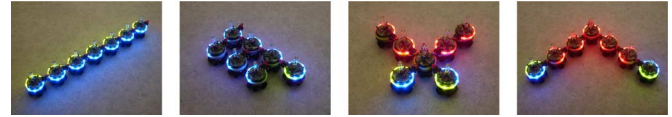
Fig. 10. Reprinted from [19]. Four morphologies grown with seven real robots: Line, arrow, star, rectangle. (The rectangle and star morphologies would become symmetric with the addition of more robots.) Videos of experiments conducted with real robots and in simulation can be found in the supplementary material online at http://ieeexplore.ieee.org or at http://iridia.ulb.ac.be/supp/IridiaSupp2008-017 .
