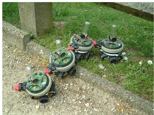
**Fig. 1** A *swarm-bot* moving in an outdoor environment. The traction system of each *s-bot* is composed of both tracks and wheels. On top of it, a rotating turret is mounted, which holds many sensory systems and the rigid gripper for physical connections
